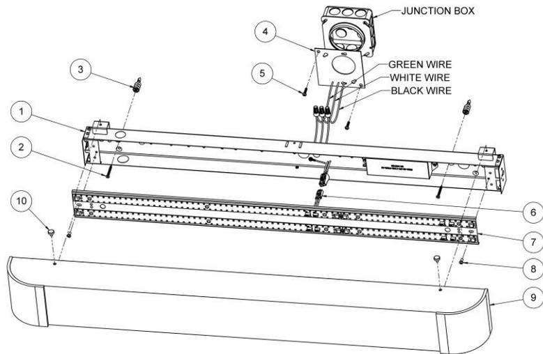
**Wiring – All wiring must take place inside junction box (not included).**
